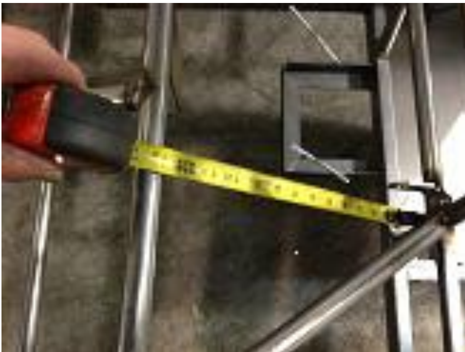
13in from upper link to petrol tank bar
