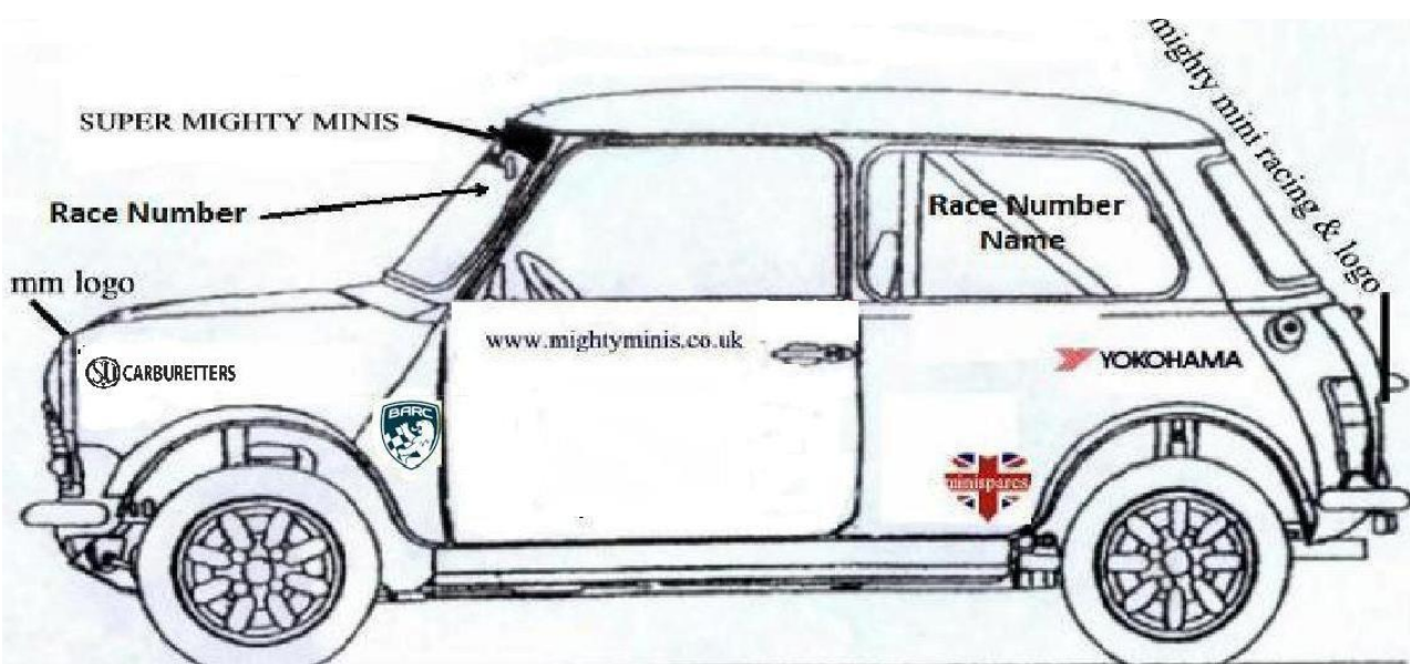
Illustration "A" . The above diagram illustrates the exact position of series sponsors' decals supplied by the organisers. These decals must be in place on both sides of the car in the positions shown, during all official practice sessions and races. This relates to Regulation 5.17.1. Additionally, one Mighty Minis logo is to be placed on the forward facing area of the bonnet, driver's side, next to the bonnet badge. Another Mighty Minis logo is to be affixed to the boot next to the badge. And the Mighty Minis Racing sticker to go below the rear no. plate
