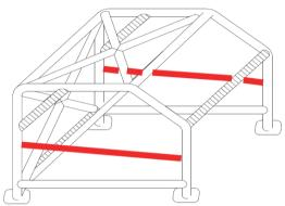
The material specification must comply with the one detailed below for the roll cage and must have a minimum diameter or side length, of 25mm.
