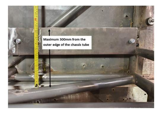
Please note the 2 images above show a Ballast Plate (SHP Part #D0825) with only 2 holes drilled. For 2020, there must be 4 holes drilled in as shown in Drawing D2 on page 32 of these regulations. Championship Regulations 5.14.1, 5.14.2 and 5.14.3 must be strictly adhered to.
