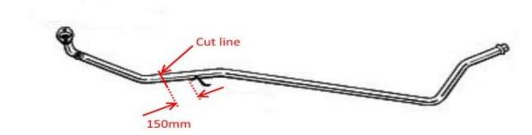
The overall length of the exhaust centre pipe must not be altered. You may either use a Universal Exhaust Pipe Sleeve Clamp as shown below or make a slip joint.
