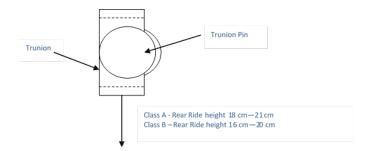
The ride height from the base of the vehicle's front sill seam (measured below the A panel to sill join) to the floor must be between 18cm and 21cm for Class A and must be between 16cms and 20cm for Class B (Tolerance 0.2cm).
