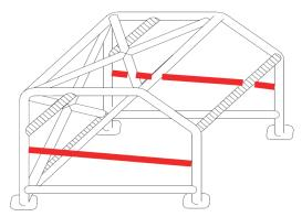
The material specification must comply with the one detailed below for the roll cage and must have a minimum diameter or side length, of 25mm.
