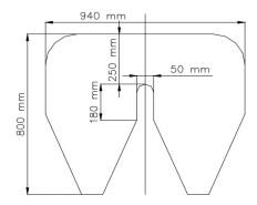
The material is free, but the fifth wheel must have a minimum weight of 5 kg.
