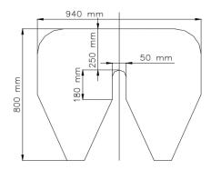
The material is free, but the fifth wheel must have a minimum weight of 5 kg.
