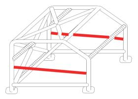
The material specification must comply with the one detailed below (see 5.3.2) for the roll cage and must have a minimum diameter or side length, of 25mm.
