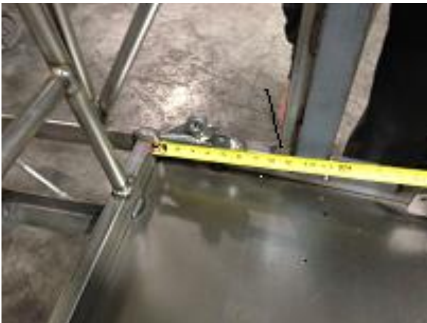
34 coupe. Rear cross to b- post Rear cross to b-post is 8in
