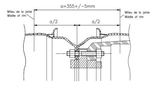
5.12.5 On rear twin wheels, the measurement 'a' must be respected in the drawing below.
