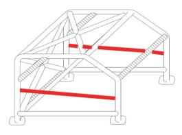
The material specification must comply with the one detailed below (see 5.3.2) for the roll cage and must have a minimum diameter or side length, of 25mm.
