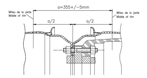
5.12.5 On rear twin wheels, the measurement 'a' must be respected in the drawing below.
