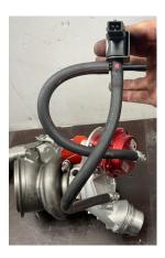
It is permitted to relocate the boost control value as shown below:
