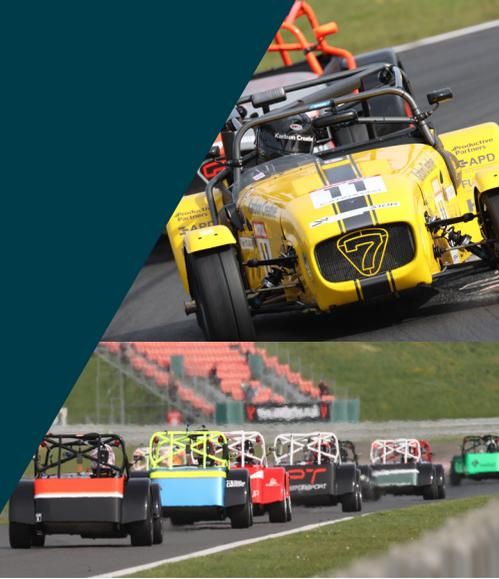
The final evolution of the Academy car, the Seven 310R looks identical to the Seven 270R, but the change in name reflects the increase in power to weight ratio, as the power is pushed up to >150bhp and a limited-slip differential is added to allow it to be exploited to the full.
